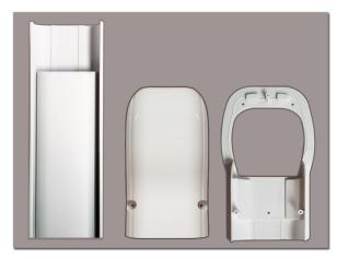
Separate the tubing and parts from front to back as the backs are installed first. Front tubing is smooth and smaller to ensure a secure fit. Be sure to keep screws with the applicable part.
